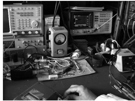
Fig. 3. A) Experimental asset. The far-field spectrum analyzer is placed on the table about 50 cm. far from the g.d.m and the passive oscillator. A small antenna picks up the r.f. field. The author right hand is moving the L/C oscillator tuning to achieve a resonance with the grid dip meter: when the resonance is achieved, the spectral line on the display is immediately depressed (B)
