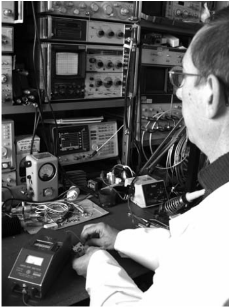
Fig. 3. A) Experimental asset. The far-field spectrum analyzer is placed on the table about 50 cm. far from the g.d.m and the passive oscillator. A small antenna picks up the r.f. field. The author right hand is moving the L/C oscillator tuning to achieve a resonance with the grid dip meter: when the resonance is achieved, the spectral line on the display is immediately depressed (B)
