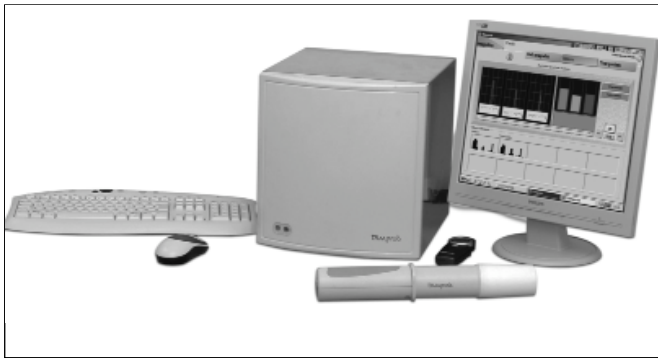
Fig. 1 - The TRIMPROB device, consisting of a battery-operated probe, a receiver and a control computer with software for data acquisition and calculation.
